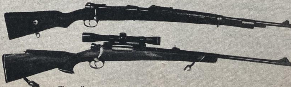
Two 8 mm model 98 Mausers. Bottom one is sporterized version made out of military rifle shown at top.
