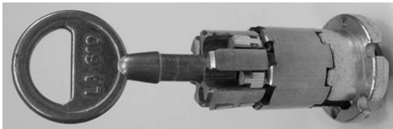
Figure 3.59: Laperche core with key inserted and pins at interface of stator ring.
