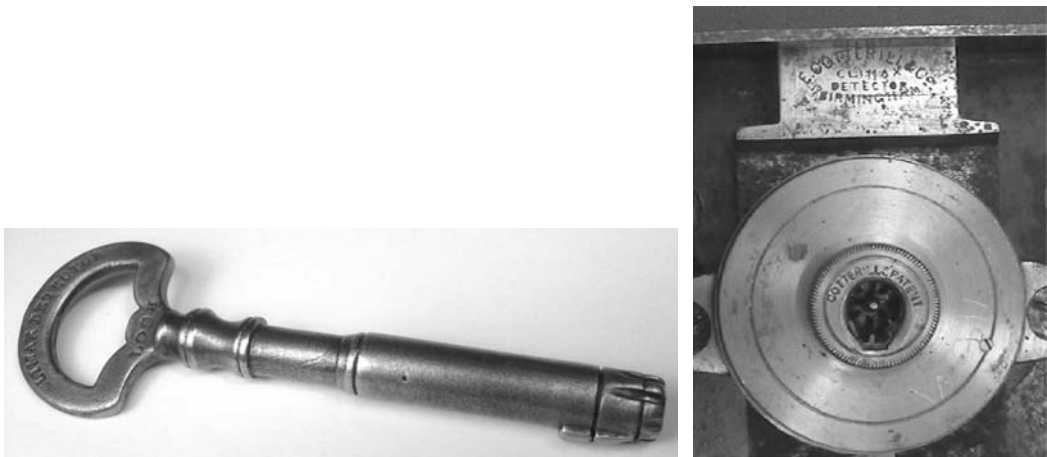
Figure 5.96: Cotterill key and 8-lever radial lock.
