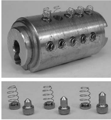
Figure 2.143: (Top) Core from BKS Janus cylinder. (Bottom) Pins, drivers and springs.
