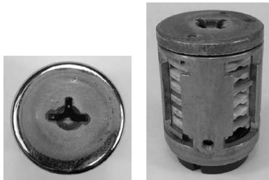
Figure 3.28: Bricard SuperSûreté 8-disc, 3-sided wafer cylinder (left); core and shell (right).
