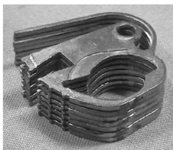
Figure 5.142: Sargent & Greenleaf 6804 levers have identical bellies and gate positions.
