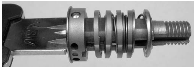
Figure 3.33: ABA plug with key fully inserted.
