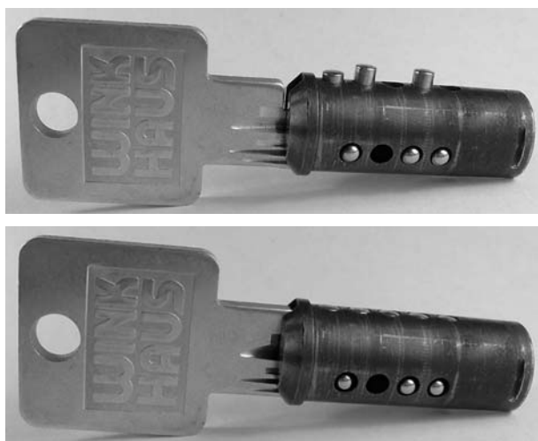
Figure 2.56: (Top) Winkhaus plug with key partially inserted. (Bottom) Key fully inserted.
