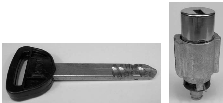
Figure 7.37: Lancia/Alpha-Romeo key and 10-pin lock barrel.
