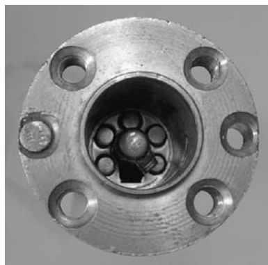
Figure 2.165: Underside of Izis cylinder with key inserted and turned.
