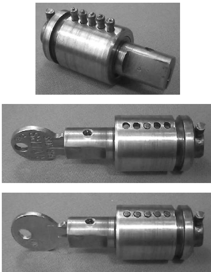
Figure 2.48: (Top) Suspended drivers leave inner core free to turn. (Middle) Incorrect key blocks outer core. (Bottom) Correct key positions pins at shear line of outer plug.
