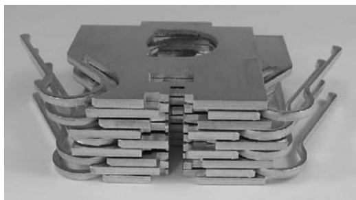
Figure 5.140: Ross 700 lever pack: (left) levers in locked position; (right) levers with gates aligned. Note: levers are identical except for gate position.
