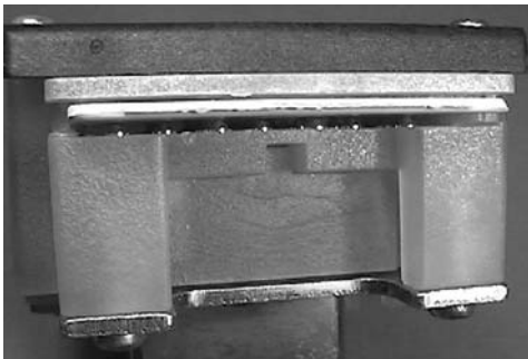
Figure 2.202: (Left) Both cards correctly inserted and carriage in open position. (Right) Pass card inserted upside down, the control card is pushed down too far.
