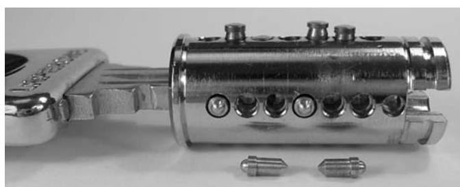
Figure 2.75: Laperche Diam 7-pin core with two passive profile pins installed. Note the spooled lower pins.
