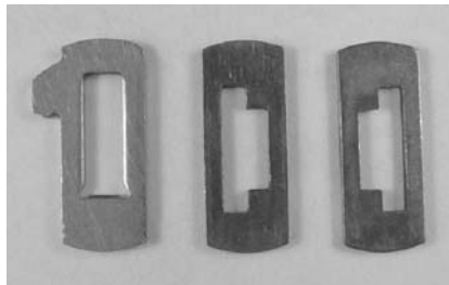
Figure 3.18: Conventional wafer-tumbler and two Bricard wafer-tumblers.
