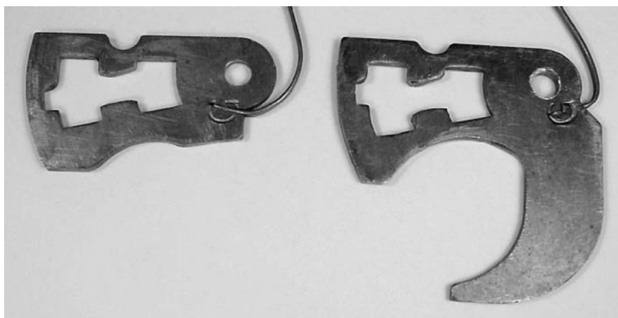
Figure 5.53: Levers from a Chubb detector lock: (left) regular lever; (right) monitor lever.
